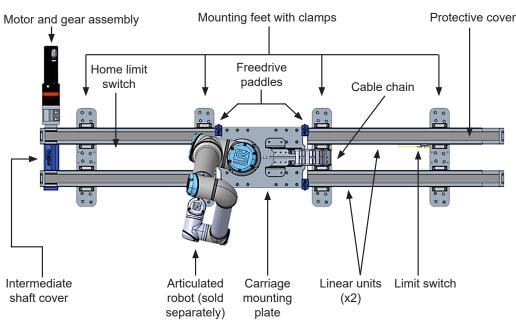
Included: Dual linear units, Kollmorgen servo motor, precision gearhead, carriage mounting plate for robot, Freedrive paddles, end-of-stroke limit switches, cable management, control box and software with 7th axis collision detection. For Universal Robots, a URCap is available for programming directly on the UR Teach Pendant.
